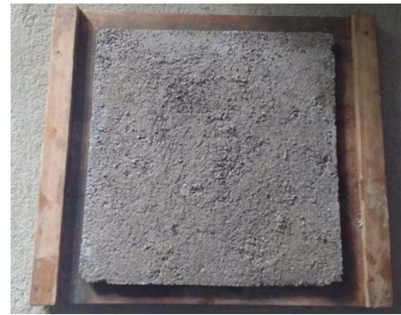
Fig. 8. – Vermiculite Tiles (304.8 mm x 304.8 mm x 304.8 mm)
