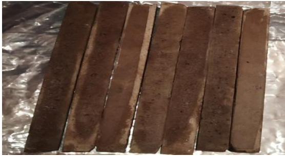
Fig. 6: Plate of finished brake pad samples
