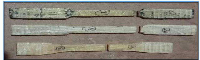
Fig. 4.2 Tested specimen on UTM machine
