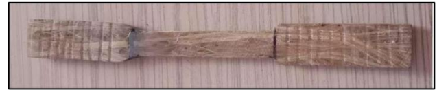
Fig. 4.1 Tensile test specimen as per ASTM E8 Standard
