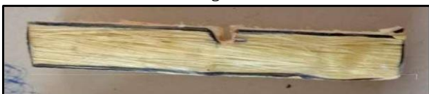
Fig. 4.7 Standard specimen of Charpy Impact Test.
