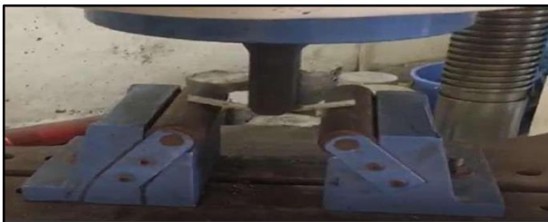
Fig. 4.6 Test set up for three-point bending
