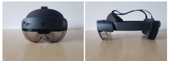
Fig. 1. The Hololens 2 optical see-through HMD
