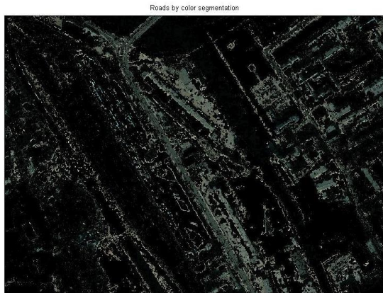
Fig 10. Output of color segmentation for roads extraction on aerial photograph 2, Phoenix city, Arizona.
