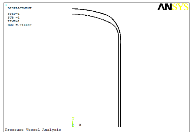
Figure 7: Deflection in baseline model of pressure vessel
