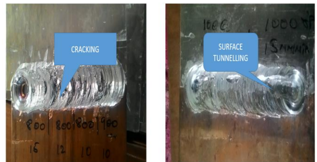
Fig 13. Defects are formed at high RPM due to this the cracking and surface tunneling is formed
