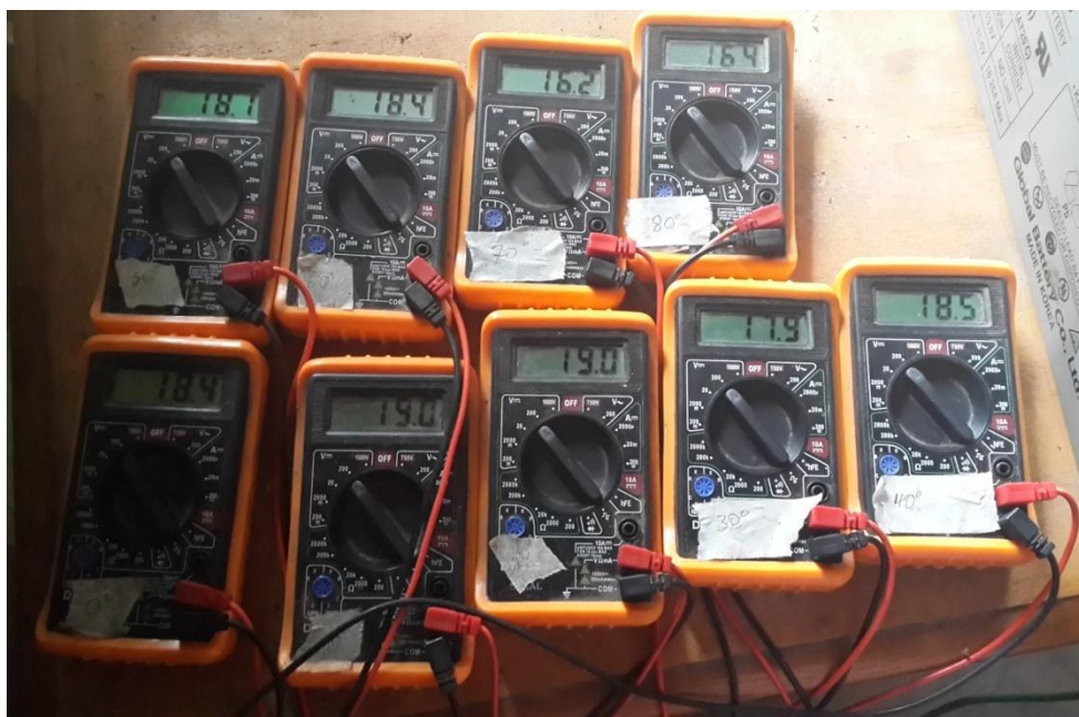
Fig. 1 Multimetre showing voltage readings of each panel
