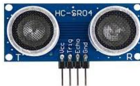
Fig 1: Layout of Ultrasonic sensor
