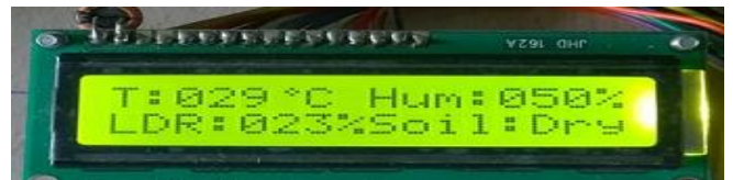
Figure No.2 16X2 LCD display
