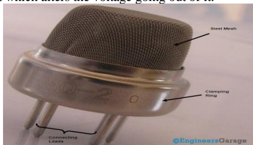
Fig. 4. Externals of a gas sensor
