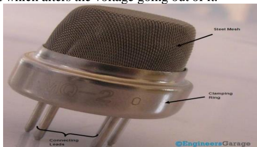
Fig. 4. Externals of a gas sensor
