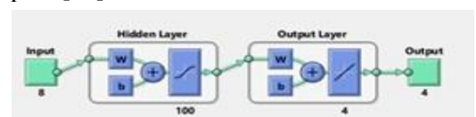
Figure (4): Fault Classifier Neural Network
