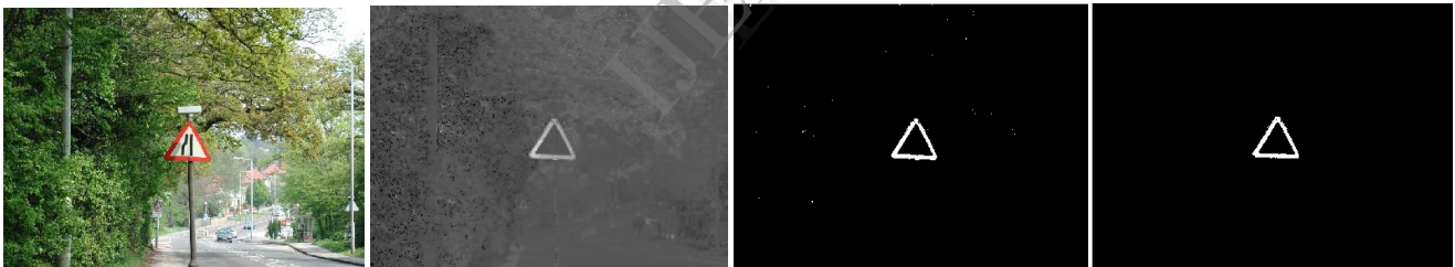
(a)Traffic sign in sunny weather (b) Normalized image (c) MSER at 'mth'= 12 (d) Binary image after area opening operation
