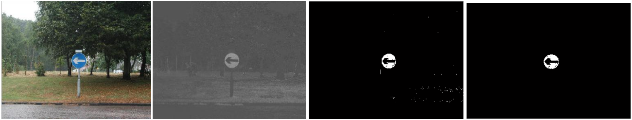
(a)Traffic sign in rainy weather (b) Normalized image (c) MSER at 'mth'= 12 (d) Binary image after area opening operation
