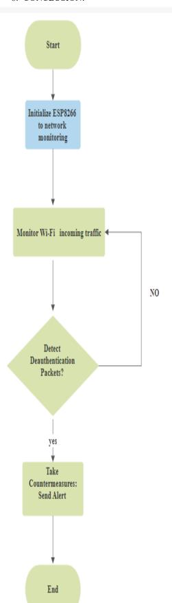
IDS offers a robust and efficient solution for identifying and reducing Wi-Fi de-authentication attacks. Here are the key takeaways:
