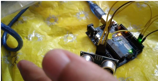
Figure 10 Ultrasonic sensor interfaced with Arduino microcontroller
