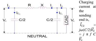
Therefore, Sending end current,  $\vec{I}_S = \vec{I}_L + \vec{I}_{C2}$
