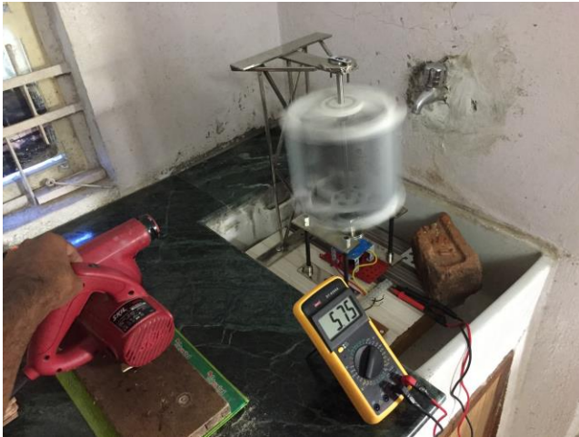
Figure 6.1- Testing with No Load
