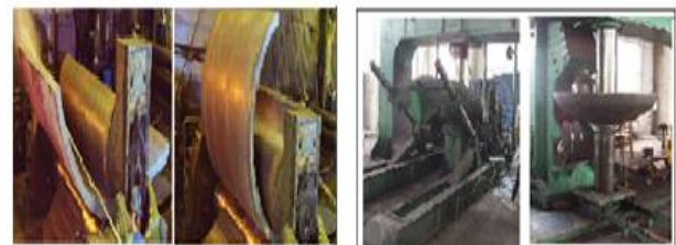
Fig 3 Shell Rolling Fig 4 head pressing to concave
