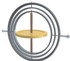
Fig.7— Gimbal with 3 axes of rotation
