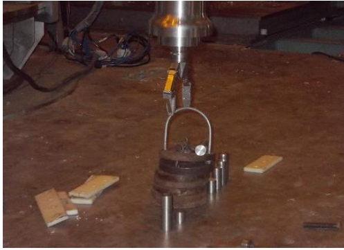
Fig.12 – PM gripper, weight 10.05kg and specimen in various lengths
