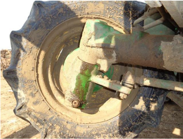
Fig.12. Field testing of axle with New Housing
