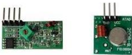
Fig. 2. RF transmitter and receiver
