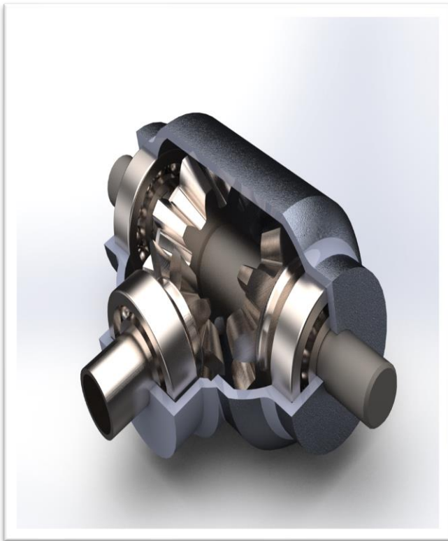
Figure 5.1 Cut section of assemblage of gear train in casing
