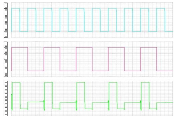
Fig.9. Simulated waveforms of SISO shift register
