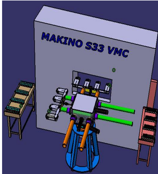
Fig.2 Pneumatic drive pick and place robot with Three-degrees-of-freedom
