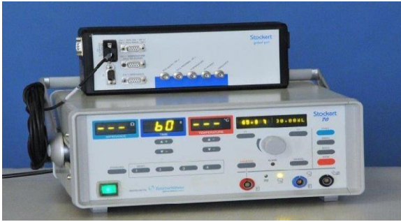
Fig. 1 STOCKERT 70 RF Generator
