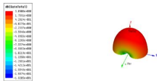
Fig. 1(c) 3D gain plot of MPA simulated using HFSS
