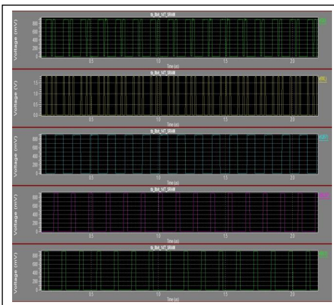
Fig. 9. Simulation waveform of 14T SRAM for 8-bit cell
