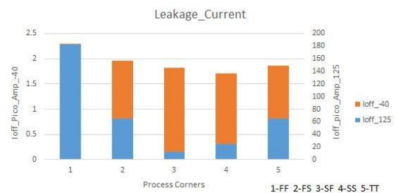
Fig. 14. Leakage Current at Standby Mode
