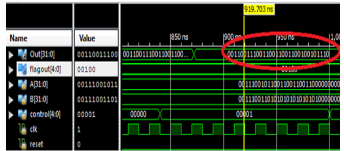
Figure 6: Simulation results Single precision floating point Multiplier
