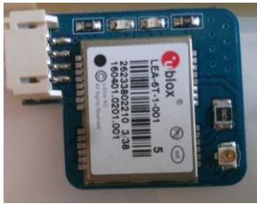
Fig.4 LEA-6T module and the GPS receiver hardware board
