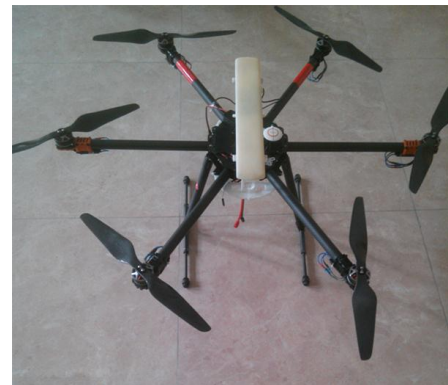
Fig.8 The six-rotor UAV test platform
