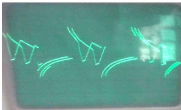
Fig. 7 Hardware simulation in oscilloscope of power inverter Using PWM pulses Continuous
