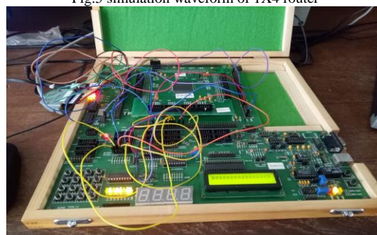
Fig. 6 Router Implementation on FPGA
