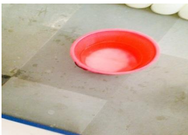
Image 4: Preparation of NaOH solution \text{Fiber-OH} + \text{NaOH} \rightarrow \text{Fiber-O}^-\text{Na}^+ + \text{H}_2\text{O}
