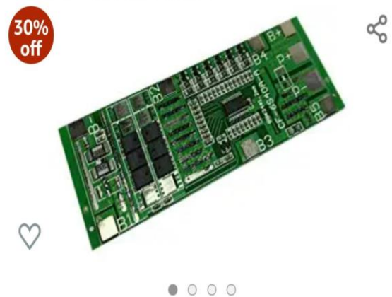
Electrobot BMS 6S 40A 24V 18650 Li-ion Li-po Battery Protection Board ebike ebicycle
