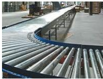
Powered roller belt type conveyor
