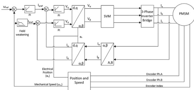
Fig-1 – Block Diagram of FOC method
