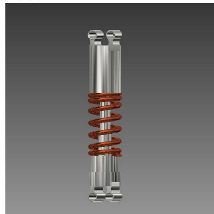
Fjg: 2.2.3 Suspension for robot arm.
