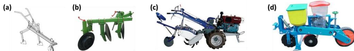
Fig. 2: Option of soil engaging components: Animal draft cultivator (a) [1]; Disc plough (b); Rotovator (c); Precision planter (d).
