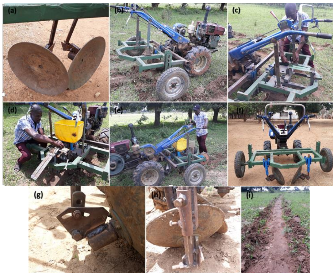
Fig. 4: Assembly process. (a) discs set facing outward for scrapping weeds before planting; (b) weeder set for weed crapping; (c) mounting of an adapter to incorporate planter components; (d) incorporation of planting components i.e. hoppers, seed metering, tines and discs on the adapter plate; (e) complete weeder incorporated with a planter; (f) discs set facing inwards for weeding after crop emergence; (g) setting of tilt angle; (h) disc angle; (i) weed-free planting strip.
