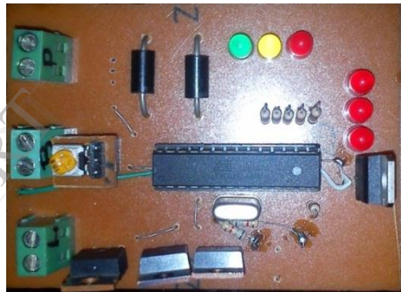
Figure 6. Actual hardware of the SCC for a 100WP SHS
