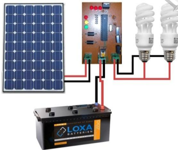
Figure 3. Charge controller and battery wiring
