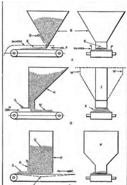
hoppers used for granular material
