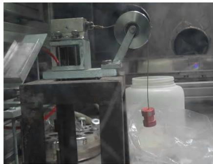
Fig. 8. Instrument for knowing the coefficient of friction between the powder particles and between the powder and the hopper material.
