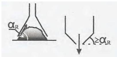
Fig. 11 Angle of repose of the powder
