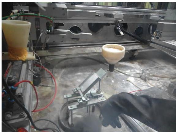
Fig. 15 Study of frictional angle between the powder and the UHMWPE hopper
