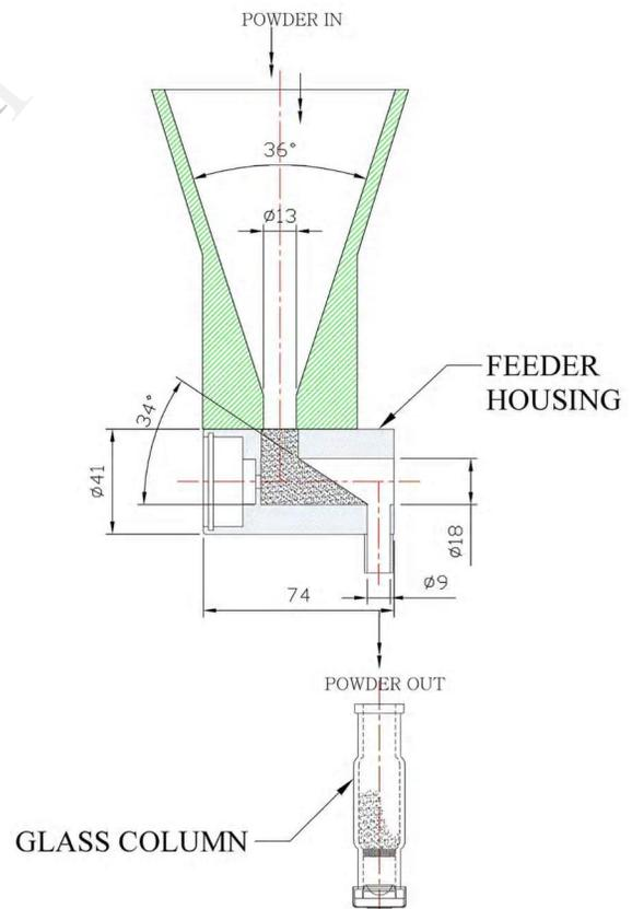
Fig. 22 Sectional view of the typical arrangement of the hopper, the powder, the spout of the dispenser and the GC.
