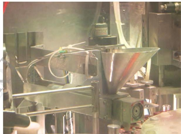
Fig. 24 Fabricated VDC SF based powder dispenser
