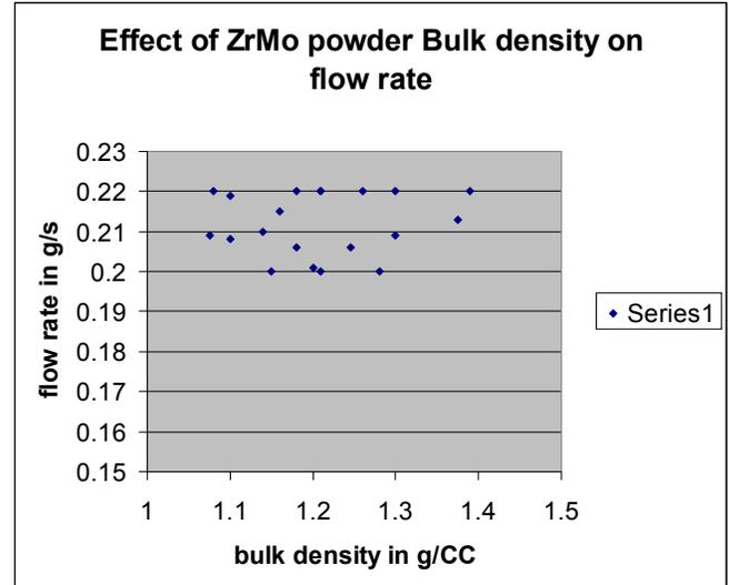
Fig. 27 Variation of the flow rate of the powder dispenser with bulk density
