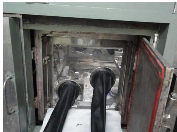
Fig. 14 Maintenance door with transparent barrier of the STB used for studying the powder properties
