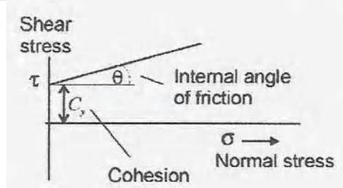
Fig. 18 Theory of internal angle of friction
