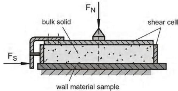
Fig. 10 Measurement Wall Friction using Jenike shear tester
