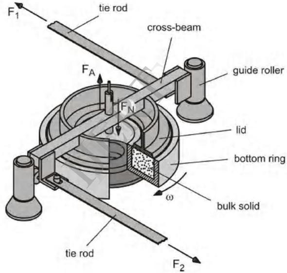
Fig. 9 Schulze Ring Shear tester
