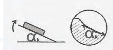
Fig. 13 Instrument for knowing the frictional angle
