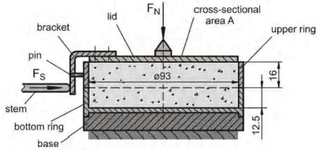
Fig. 8 Shear Cell of the Jenike Shear Tester
