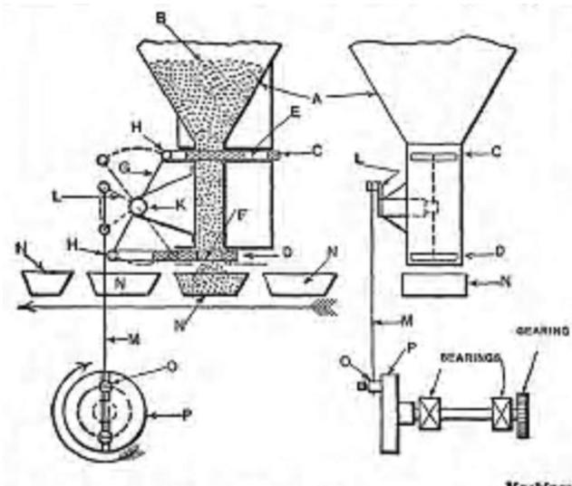
Fig.6 Hopper valves arrangement for handling granular substances
