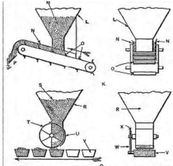
Rotating hopper valve mechanism
