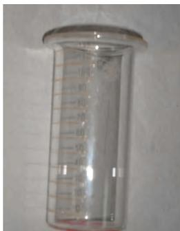
Fig. 7. Metering beaker to know the volume of the untapped Zr-Mo powder produced
