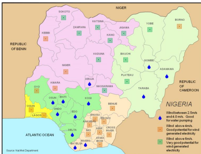
Fig. 3: wind energy potential in Gusau, Zamfara state and other states in Nigeria [5]
