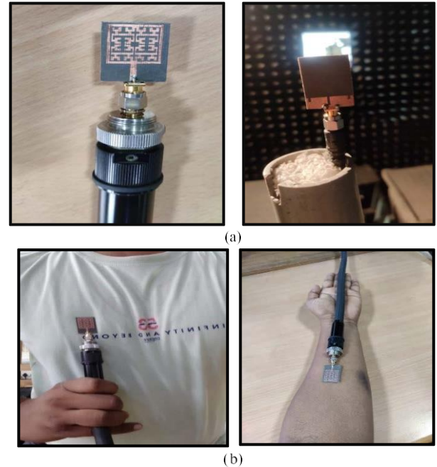
FIGURE 9. Antenna under measurement a) in anechoic chamber b) Placement of antenna over different parts of the body.
