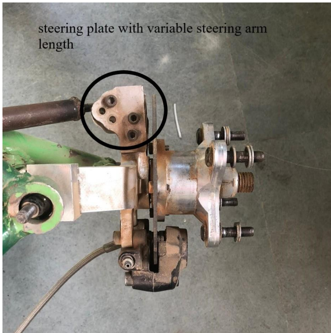
Fig 6 shows variable steering arm length plate
