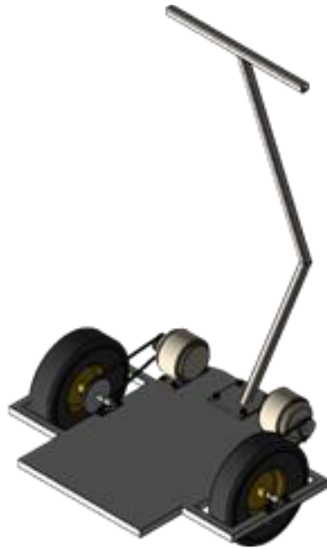
Fig. 10 Basic Design for Making the Mechanical Hoverboard
