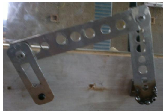
Fig.2. Assembly of holed Wiperlinks
