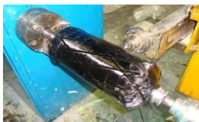
Fig. 5 Filament winding over liner
