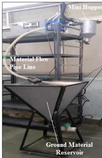
Fig 1. Experiment set up of Flexible Hopper Feeding Mechanism.
