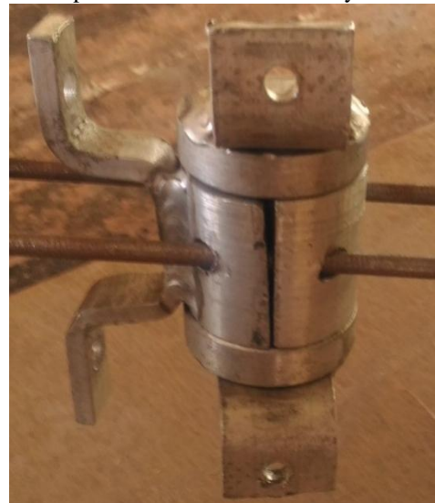
Figure 5 Manufactured Hinge Part
