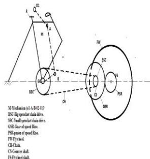
Figure. Side view for Human Powered Flywheel Motor divided in to three subsystem (i) Energy Unit: Comprising of a suitable peddling mechanism, speed rise gear pair and Flywheel conceptualized as Human Powered Flywheel Motor (HPFM) (ii) Suitable torsionally flexible clutch and torque amplification gear pair and (iii) a process unit. Essentially the flywheel motor consists of flywheel, which is being driven by a human
