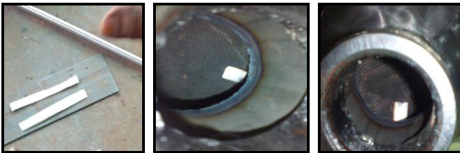
Fig. 9: L-Clamps, (A) Strips to make Clamps (B) & (C) Welded L-clamps to Support wire Mesh Substrate
