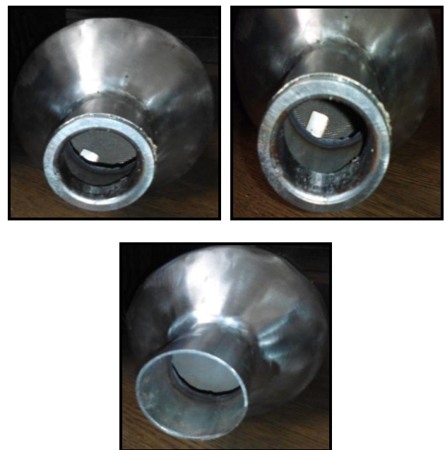
Fig. 13: Tapping's, (A) Inlet Tapping (B) Coupler glued at Inlet & L- clamp to support wire Meshes (C) Exhaust Tapping
