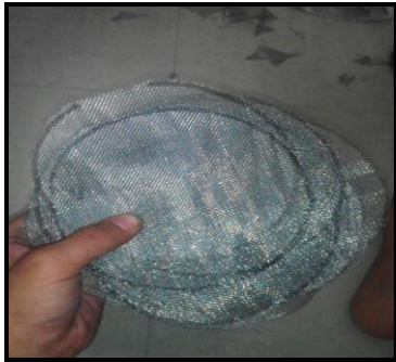
Fig. 5: Wire Meshes acting as Catalyst Substrate
