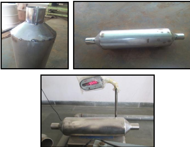
Fig. 10: Welding, (A) Spot Welding done to form Tapping (B) Completely Spot Welded Prototype (C) Finished Prototype with Weight
